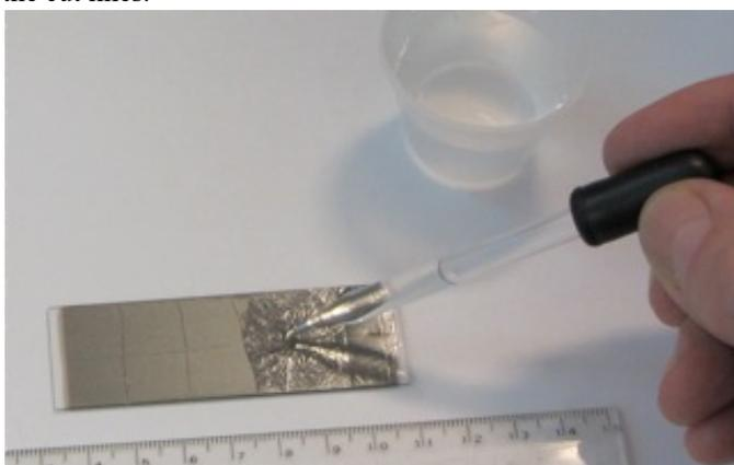
Fig. 8a. Floating a foil by immersing its substrate by hand, into a water bath. The foil in this photo is on a glass slide; the slide is held with forceps:
