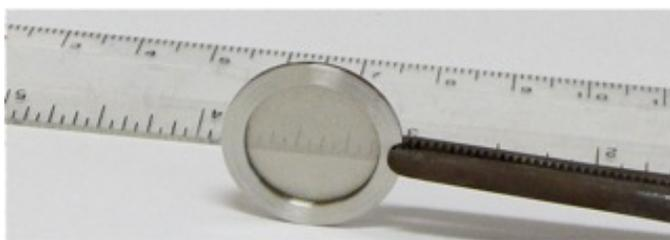
Fig. 5b. Evaporated carbon foils mounted with free edges, approx. 75 µg/sq.cm on cyclotron forks F30 (left) and F12 (right, in plastic cell).
