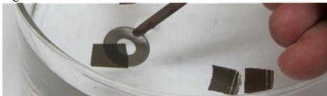
Fig. 9b. The frame is pressed against the piece of foil so that the foil drapes over the aperture to be covered, and then is raised slowly. The foil usually adheres to the exposed surface of the frame.
