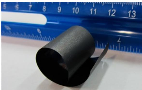
Fig. 4: Evaporated carbon foil, approximately 1.5 microns' thickness (300  $\mu\text{g}/\text{sq.cm}$ ), removed from substrate without annealing. The radius of curvature in this example is approximately 1 cm.
