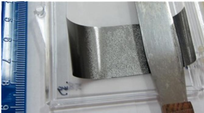
Fig. 3. Evaporated carbon foil (approx. 100  $\mu\text{g}/\text{sq.cm}$ ) on glass substrate 25 mm x 75 mm, showing compression-wrinkle pattern due to internal stresses (see section 2.5 below). This particular foil's substrate is glued permanently into its transparent plastic shipping box. This foil can be removed from its substrate by slowly immersing the substrate and box in water (see section 2.22 below).
