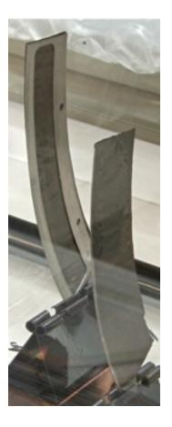
Methods #2, #3, and #4 require the foil to flex only in one direction, important for minimizing cracks. When a suitable rate of release is found, it is desirable to maintain the release rate as constant as possible until the foil has been completely released. In every case, a light-colored background helps to make the foil clearly visible.
