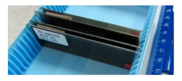
Fig. 2. Evaporated carbon foil (approx.  $80 \mu g/sq.cm$ , 25 mm x 68 mm) removed from its substrate. The tendency to curl indicates residual stresses in the foil (see section 2.5 below):
