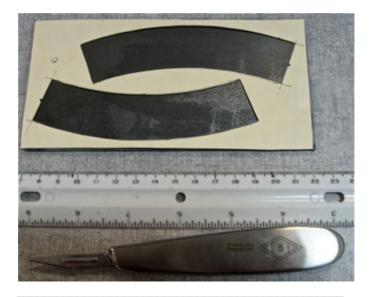
Note that for any of these techniques, if the floating process is interrupted, and the partially released foil is allowed to reattach itself to its substrate, and/or if the parting agent under the unreleased part of the foil is recrystallized by the high humidity near the water surface and then dried, the foil may not release later.
