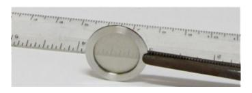
Fig. 5b. Evaporated carbon foils mounted with free edges, approx. 75  $\mu$ g/sq.cm on cyclotron forks F30 (left) and F12 (right, in plastic cell).
