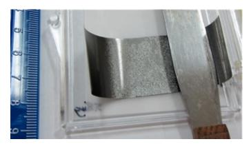
Fig. 3. Evaporated carbon foil (approx. 100 µg/sq.cm) on glass substrate 25 mm x 75 mm, showing compression-wrinkle pattern due to internal stresses (see section 2.5 below). This particular foil's substrate is glued permanently into its transparent plastic shipping box. This foil can be removed from its substrate by slowly immersing the substrate and box in water (see section 2.22 below).
