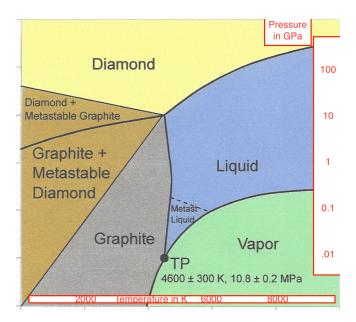
Figure 9d: Theoretical carbon phase diagram from [Wikimedia (2017)]. Note that this reference claims that considerable disagreement exists between theory and experiment.
