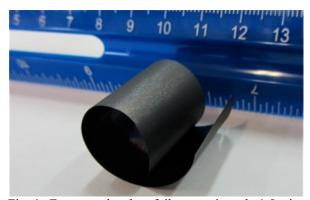
Fig. 4: Evaporated carbon foil, approximately 1.5 microns' thickness (300  $\mu$ g/sq.cm), removed from substrate without annealing. The radius of curvature in this example is approximately 1 cm.
