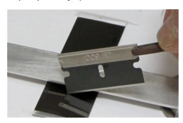
If the foil has started to release from its substrate, do **not** use a single blade to cut it on its slide; the foil may splinter where it is cut. Either use a double-blade method, in which one blade reduces the spread of damage due to cutting (Fig. 6b below), or use a method described in Sections 2.20 and 2.21 below. Float it and pick it up in the usual manner (see below).
