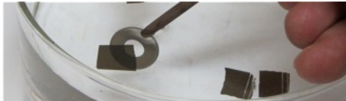
Fig. 9a Typical pickup sequence for foil onto washer used as a frame. A piece of foil is sequestered, preferably near the edge of the water surface.
