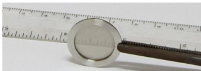
Fig. 5a Evaporated carbon foil, approximately 5\ \mu\text{g}/\text{sq. cm} , on 70 line-per-inch mesh on mounting ring.
