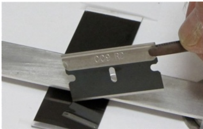
Fig. 6a Cutting a foil on its glass substrate, using a single razor blade. The straightedge is supported above but not touching the foil, and both straightedge and foil are clamped or taped in place for rigidity.
