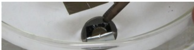
Fig. 9b The frame is pressed against the piece of foil so that the foil drapes over the aperture to be covered, and then is raised slowly. The foil usually adheres to the exposed surface of the frame.
