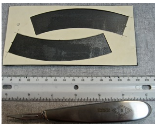
Fig. 8c A cardboard mask is used to guide a scalpel blade for cutting the desired foil pieces. The foil is then placed on its support in the lower aquarium.
