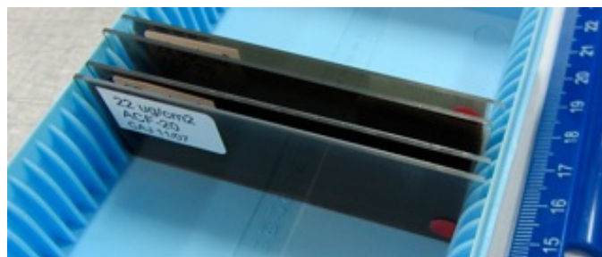
Fig. 1 Evaporated carbon foils (approx. 22 \mu\text{g}/\text{sq.cm} ) on glass substrates 25mm x 75mm.
